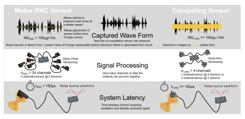
excitation and the processing unit receiving the signal, which means the noise is cancelled more efficiently. Plus, the sensors can measure road noise at slower speeds and be placed farther away from the sound source, while providing more network data channels as well.
