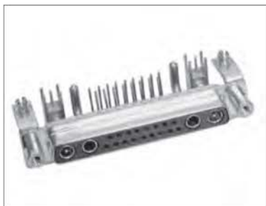
Fig. 1: Mixed Layout socket connector, contact arrangement 21WA4, 2 high power and coaxial contacts with right angled PCB termination and several accessories
