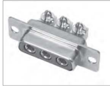
Fig. 3: Mixed Layout socket connector, contact arrangement 3W3, 3 high power contacts with right angled PCB termination in press-fit version
