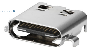
USB 3.2 Gen 1 Type-C Receptacle, Mid-Mount, 24 Circuit (217184 series)
