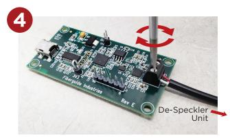
Hold each wire in place and screw down the screw in the terminal block to clamp the wire and form the appropriate electrical connection. Then, insert the De-Speckler into your laser pig-tail system via the fiber connectors.
