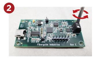
Loosen the screws on the terminal block.
