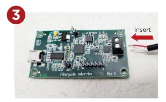
Slide the stripped region of each wire between the screw and the base of the component: the red wire in the + position, and the white wire in the - position, as indicated on the PCB.
