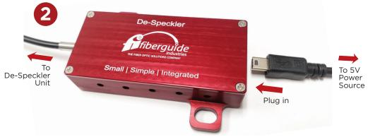
Connect a USB Mini-B cable (USB-A termination) to a 5 Volt power source such as a computer USB port or a plug-in outlet converter. Then, insert the De-Speckler into your laser pig-tail system via the fiber connectors.
