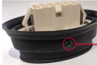
Lock nails not visible
