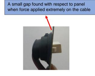
This case is not taken into consideration since external factors such as bending or deforming of the wires are recommended 1 inch away from the end of the housing (PS) Refer below section
