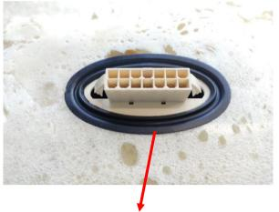
No leakage found on panel side of the housing
